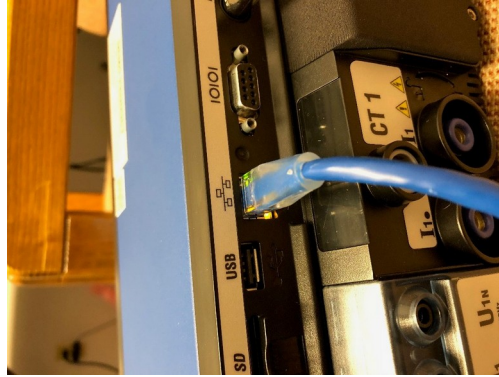
Ethernet port on the back of an RX standard.
