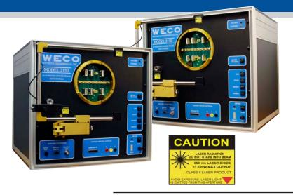
WECO's Model 2150 automated test system is a fully ANSI compliant testboard that uses a single voltage and three independently controlled isolated current sources to test all electromechanical and solid state meters up to 50 Amps. The internal NIST traceable Radian Research RD-20 series reference standard brings unparalleled accuracy.
