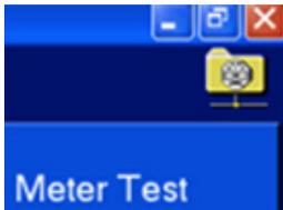
Once the Icon Appears, the Bantam Plus/WE20 has connected to the WATT-Net database on the field PC.
