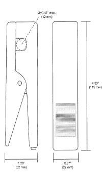
The RC-MN106 is a MN106 AC current probe manufactured by AEMC<sup>R</sup> Instruments then modified by Radian Research, Inc.
