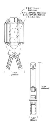
The RC-JM830A is a JM830A AC current probe manufactured by AEMC® Instruments then modified by Radian Research, Inc.
