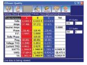
Retrieve data on the calculated electrical quantities for transformer secondaries and primaries of the meter installation with the RW-3X NS's Secondary and Primary Checks Everything from Volts to VARS is measured, in real time, across all three phases for each check. Results are clearly displayed in a color-coded table and can be changed from real time to a snapshot with the click of the stylus.
