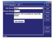
Site Information allows you to set up and recall specific information on the devices at a test site such as meters, current transformers and potential transformers. This method of data management keeps you from having to enter information while out in the field. If data is changed in the field the RW-3X NS updates the site information database so it's saved for the next time you test the site.
