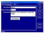
Site Information allows you to set up and recall specific information on the devices at a test site such as meters, current transformers and potential transformers. This method of data management keeps you from having to enter information while out in the field. If data is changed in the field the RW-3X updates the site information database so it's saved for the next time you test the site.
