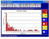
The system's powerful Harmonic Analysis feature displays harmonic data (both RMS and percent of fundamental) for all three phases up to the 60th harmonic as a bar graph or raw numbers.
