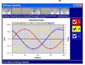
Waveform analysis gives you the ability to view voltage and current waveform graphs for all three phases. You can view a real time waveform graph for any combination of phases. The interactive graph allows you to zoom in and out as well as retrieve exact numerical measurements by clicking on any point.
