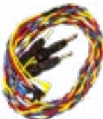
(BW0149) RW Braided 'A', 'B', 'C' Phase Current Cable Set with Saf-T-Plugs ---- The current cable set with Saf-T-Plugs connects the RW to the test switch allowing you to read the secondary current of the transformer as well as burden test the current circuit. This is a braided, 3 color-coded (red, yellow, blue) 8 ft cable.
