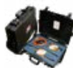
(AW0011) RW High Voltage **Current** Probe Kit, 2000 Amps, 150kV ---- The high voltage current probe kit includes a fiber optic isolated current probe with 3.85" wide jaw for current measurements of primary conductors above 600V to 150kV. Use to test CT Ratios. Detachable line hanger, adapter and probe with hot stick mounting capability all come in a convenient carrying case.
