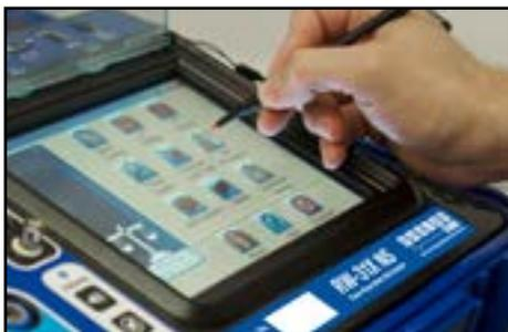
real-time. Analyze Harmonics through the 60th order providing total harmonic distortion with the amplitude and phase of each Harmonic. With Meter Testing use the customer's load for verifying meter accuracy. Transformer Testing provides burden and ratio accuracy measurement for both current and potential transformers along with demag for Current Transformers.
