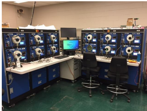
Figure 6 Light Node Testing using WECO 8000 2
