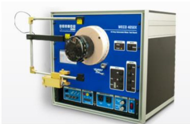
Figure 7 Light Node Testing using WECO 4050XT
