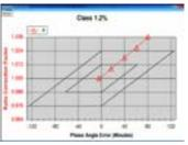
Transformer Testing allows for the selection of any combination of ratio measurement and burden testing up to a maximum of 4.0 Ohms. Selected tests automatically run through in a single pass. Numerical results are given which are also plotted on a parallelogram. A separate "Demag" process can be run to demagnetize the transformer under test.
