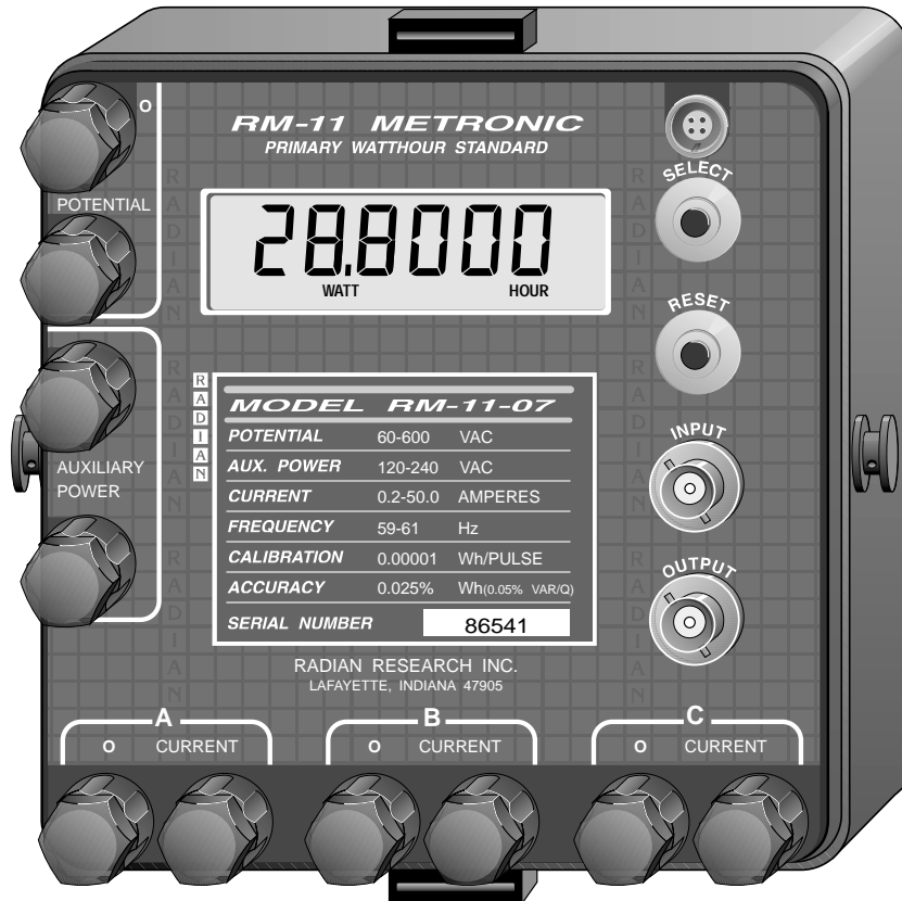
Figure 2.1 RM-11 Metronic Primary Watthour Standard
