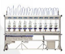
The suspension rack is constructed from light, corrosion-free and rigid aluminium profiles, so it is easy to assemble and disassemble. The standard version is available in 3, 5, 10, & 20 position options. Modular construction allows assembly for any number of test positions as per customer requirements. The SR is equipped with a photoelectric scanning heads and error calculator/indicator at each test position.
