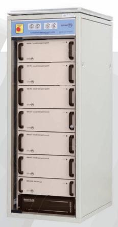
The power stage of the source (VIS & CIS) utilizes the PWM technology and is driven by an on-board DSP signal generator. The internal DSP-controlled digital feedback loops and advanced algorithms ensure quick setting, high stability and very low distortion in output current and voltage signals. The system allows users to set the phase angles and harmonics in each channel required for testing. The output voltage & current are independent from each other, isolated and free from mains supply.
