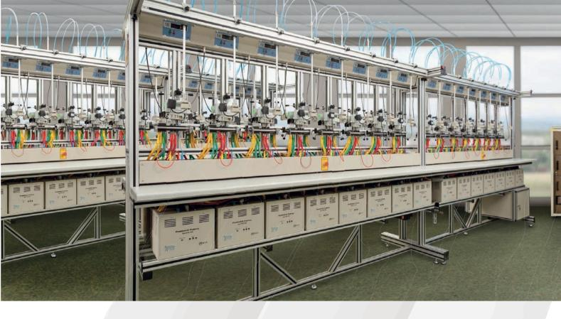
The ASTeL meter testing system is a fully automatic multi-position test system which performs the adjustment and calibration of single- and two- and three-phase energy meters simultaneously. Use of latest digital signal processing, high precision signal synthesis and quality makes the system suitable for testing a multitude of electric energy meters available in the market, from simple electromechanical devices to modern smart meters.
