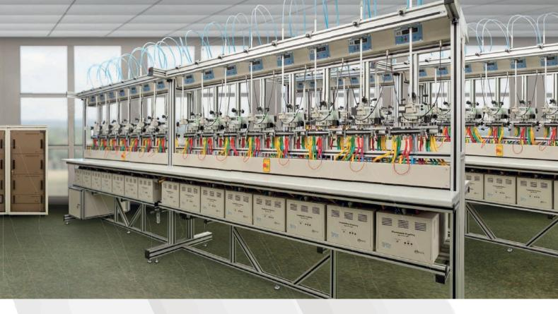
The ASTeL metering testing system is ideally suited for testing a wide range of electronic and electro-mechanical meters, as per IEC and other relevant standards and norms:
